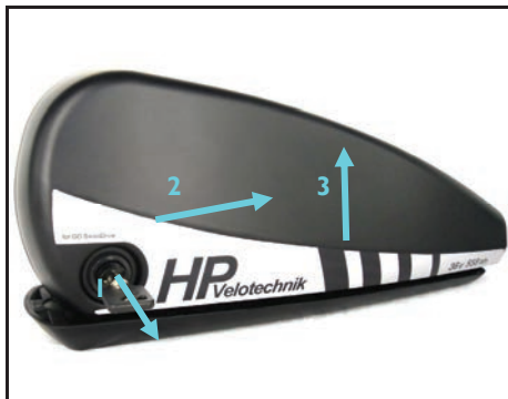
Picture 26: Removing the battery from the battery mounting rail
