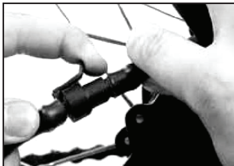
Picture 22: Disconnecting the motor connector
